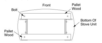
Figure 8 - Removing Pallet Wood From The Bottom of The Stove
